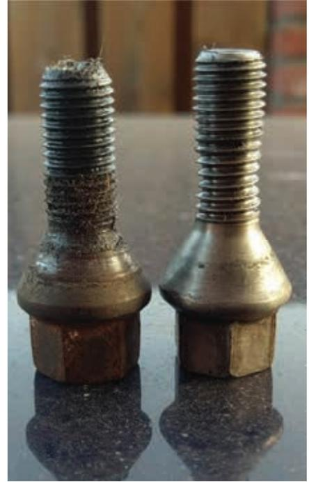
The HYTORC Gall-Free Nut coated thread design eliminates the microscopic material corrosion that occurs when fasteners are subjected to high temperatures and increased friction over extended time periods. This technology counters the galling effect of plastic deformation and micro-scale material transfer of thread surfaces.
